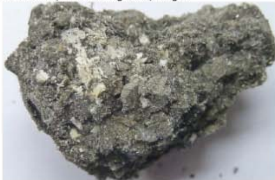
Plate 5. Intact piece of mortar containing an abundance of shell, unburnt, partially burnt and as lime inclusions.
