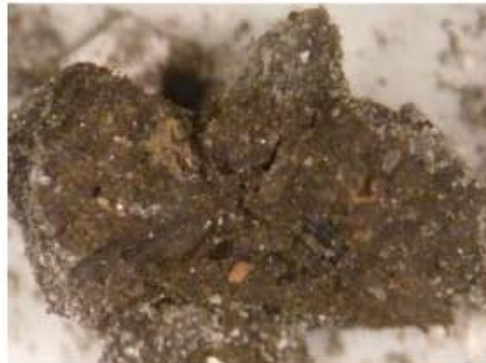
Plate 6. Intact piece of clay rich mortar encapsulating a piece of charcoal.
