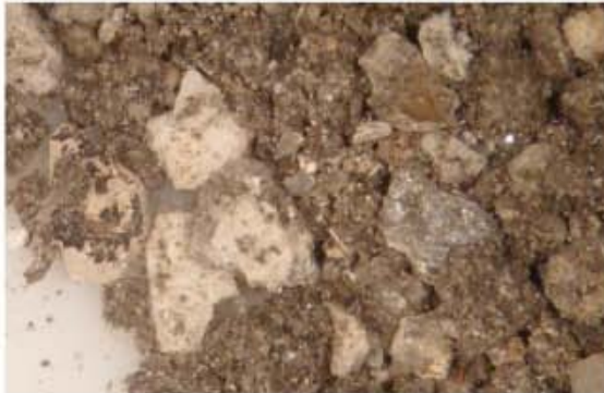
Plate 3. View through the microscope showing lime inclusions, left of centre, with shell fragments, to right.
