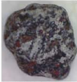
Plate 5. Grain retained in the 2mm sieve showing a notable red mineral.
