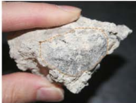
Plate 3. A broken face of the sample revealing the large granitic pebble within the mortar (highlighted by dotted line).
