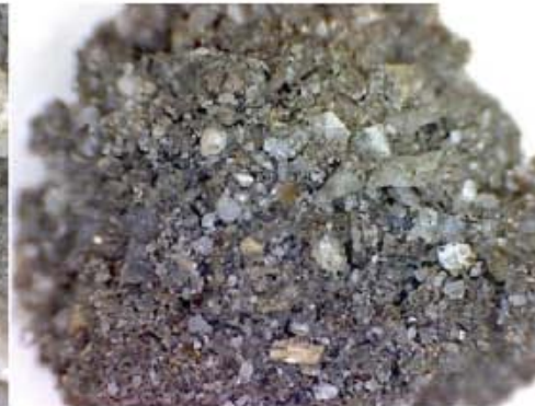
Plate 4. A small intact piece of mortar under the microscope (c. x20 magnification).
