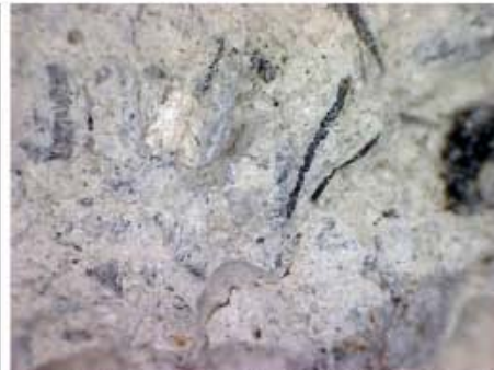
Plate 4. Close-up image of freshly broken surface of the sample (c. x30 magnification).
