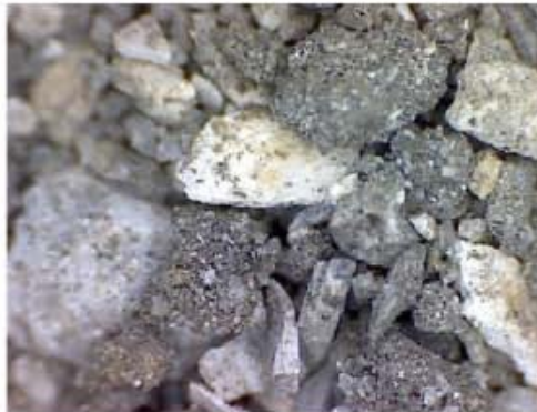
Plate 3. Some of the mortar fines under the microscope showing a white shell-lime fragment in the centre of the image (c. x20 magnification).
