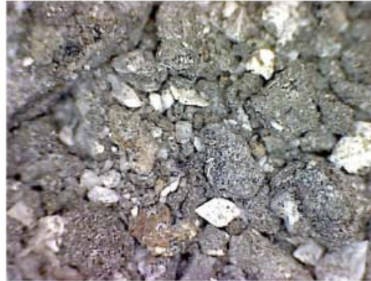
Plate 4. Close up of some of the mortar fines received (c. x30 magnification).
